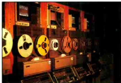
Modern analog one-inch tape machines offer high-quality signals at a low cost of operation.
